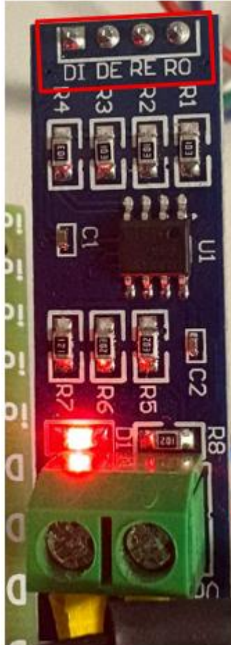
Figure 2: 4 pins that need to be set up on STEMSEL board on the Modbus board
